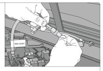
**Step 5:** Remove the terminating resistor and then plug it into the mating end of the HRN-CE10A2. Connect the HRN-CE10A2 to where the terminating resistor was removed.
