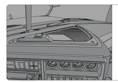
**Step 1:** Remove the three T-25 screws holding the fuse box cover in place, then remove the cover.
