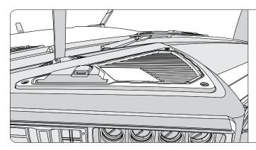
**Step 8:** Clean up all wiring using zip ties. Be sure not to obstruct any fuses. Complete an installation check for the GO device and then reinstall the fuse box cover.
