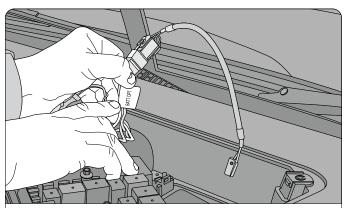
**Step 3:** Connect the 2-pin black power T-cable from the kit to the 2-pin power connector labeled BATT OPT.
