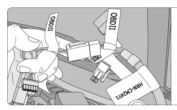
**Step 6:** Connect the 6-pin white Molex connector on the HRN-CE10A2 to the 6-pin white Molex connector on the HRN-CM24Y1. They are both labeled OBDII.
